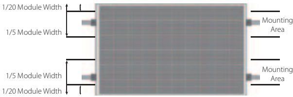
Figure3. Mechanical dimensions when modules installed in landscape orientation with clamp fitting method
