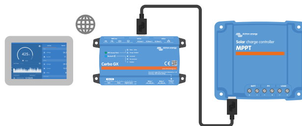
VictronConnect App connection via LAN or the internet (VRM portal) using a GX device (for example a Cerbo GX)
