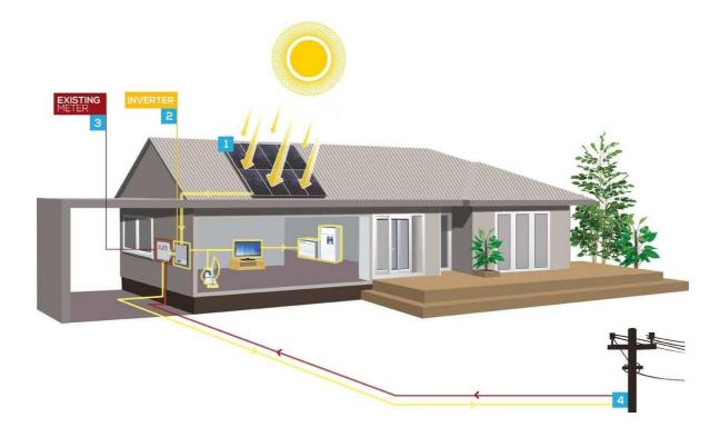
Please note that the inverter includes safety protection devices, which will isolate your solar system, should the grid voltage or frequency fall outside a specific range. This feature protects the inverter from grid spike or surges and also protects the grid line workers who may periodically need to carry out maintenance work on nearby power lines.
